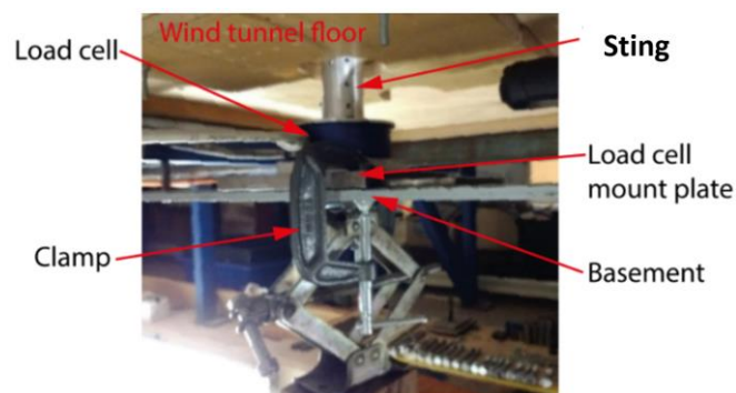
Figure 3-26: The load cell installed under the floor of the wind tunnel
