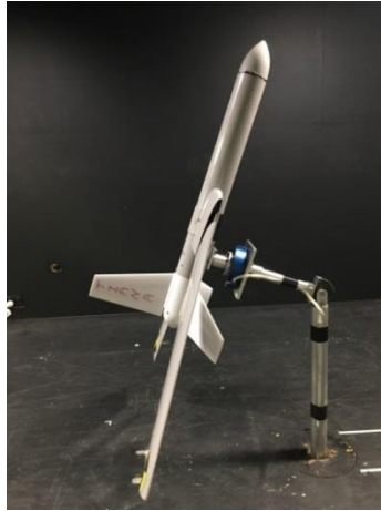
Figure 3-34: Placement of the vehicle for verifying the wing-deployment mechanism
